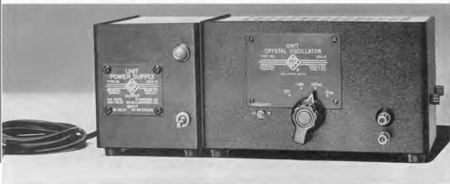
Figure 1. Panel view of the Type 1213-A Unit Crystal Oscillator with the Type 1203-A Power Supply. The two units bolt together to form a compact, rigid assembly.
