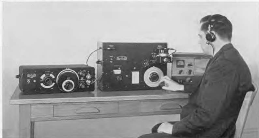
Figure 1. Setup for one-megacycle dielectric measurements. Shown are the Type 716-CS1 Capacitance Bridge, Type 1690-A Dielectric Sample Holder, and Type 1330-A Bridge Oscillator.
